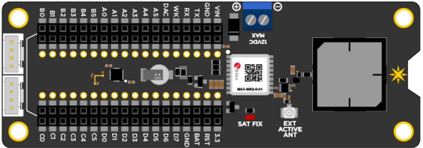
This new revision of the Electron Asset Tracker uses a uBlox M8 engine GNSS receiver. Unlike the v1, this module is capable of receiving 3 GNSS (GPS, Galileo, GLONASS, BeiDou) concurrently. We have also added a low noise amplifier and a band pass filter for improved performance with the on-board antenna.
