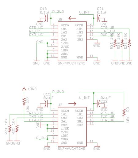
Since u-blox module's communication interface operates at 1.8VDC, while the STM32F205RGT6 microcontroller operates at 3.3VDC, we need voltage translators in-between them. This is achieved with two SN74AVC4T245 non-inverting buffers. The default state of the USART pins is set with the help of pull-up and pull-down resistors, and the unused input pins are tied to GND.
