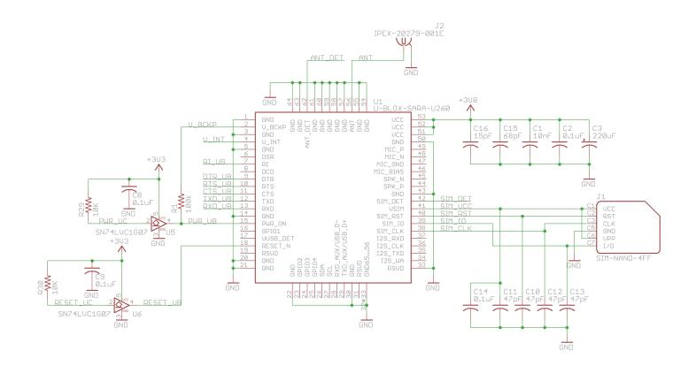
The u-blox cellular module talks to the microcontroller over a full-duplex USART interface using a standard set of AT commands. The SIM (Nano 4FF) card is directly connected to the u-blox. The power to the SIM card is also provided by the cellular module.
