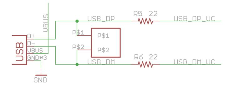
The USB data lines are terminated with 22 Ohm resistors. These data pins are also exposed via small through holes next to the USB connector and are labeled D+ and D-. The VBUS (+5VDC VCC of the USB port) is fed to the PMIC via a 3Amp Schottky diode (SS3P3). The VBUS pin is also available via the unpopulated header hole on the top-right side of the Electron.
