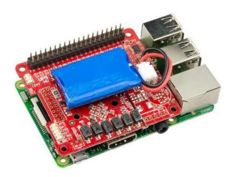
The **UPS Pico HV3.0B Stack 450** is an advanced uninterruptible power supply for the Raspberry Pi A+/B+/2/3, that adds a wealth of innovative power back-up functionality and development features to the innovative microcomputer! The UPS Pico will automatically shut-down your Raspberry Pi if there is a power failure, and can be set to automatically monitor and reboot your Pi once power has been restored!
