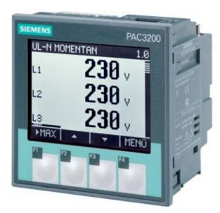
SENTRON, measuring instrument, 7KM PAC3200, LCD, L-L: 690 V, L-N: 400 V, 5 A, 3-phase, Modbus TCP, optionally Modbus RTU / PROFINET / PROFIBUS, apparent / active / reactive energy, class 0.5 according to IEC61557-12 or Class 0.5S according to IEC62053-22, wide voltage range power supply unit, AC/DC, screw terminal
