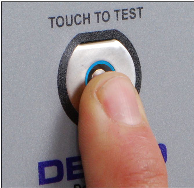
Figure 10. Bridging the test switch's contacts to initiate the test
