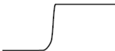
Signal with a short length ground lead
