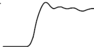
Signal with a long ground lead
