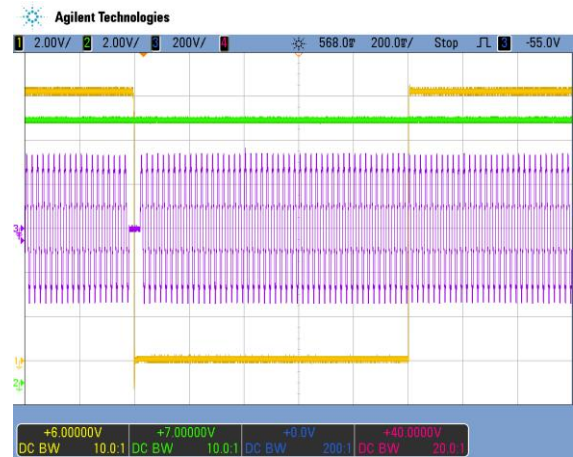
Figure 14 - AC drop out 40 ms, full load (200 ms/div), V1 restart after 1 sec CH1: V1 (5 V/div); CH2: VSB (2 V/div); CH3: I1 (200 V/div)
