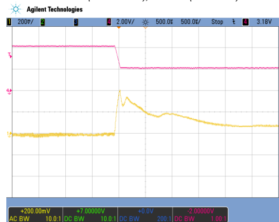
Figure 18 - Load transient V1, 244 to 122 A (500 \mu s/div) CH1: V1 (200 mV/div); CH4: I1 (100 A/div)
