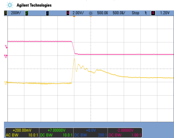
Figure 16 - Load transient V1, 125 to 3 A (500 \mu s/div) CH1: V1 (200 mV/div); CH4: I1 (100 A/div)
