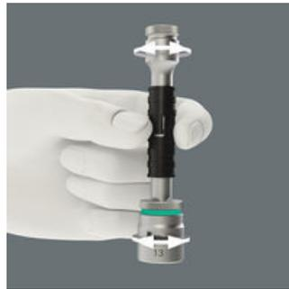
The extensions from the premium lines are also equipped with the unique "flexible-lock-system". By activating this system, attachments can be fixed to the extension permanently – preventing slipping and any unintentional loss of the attachment. When the system is deactivated, the sockets can be attached as usual and changed in a flash.
