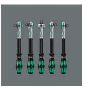
The ratchet head pivots freely and can be locked into any position by using the slide switch that is positioned on either side. It is even possible to work in very confined and difficult-to-access areas with enhanced hand clearance. The predefined locking at 0°, 15° and 90°, both to the right and left, ensure safe working without any slipping of the ratchet head.
