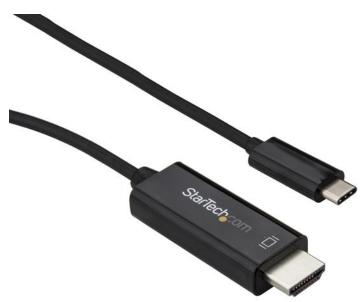
This USB-C<sup>™</sup> to HDMI® adapter cable offers a convenient solution for directly connecting your DisplayPort over USB Type-C<sup>™</sup> device to your HDMI monitor, television, or projector. The adapter offers a connection distance of up to 3 m (10 ft.) and works with USB-C devices that support DP Alt Mode, such as the MacBook, Chromebook Pixel<sup>™</sup> and Dell<sup>™</sup> XPS<sup>™</sup> models 15 and 13. It's also compatible with Thunderbolt<sup>™</sup> 3 ports.
