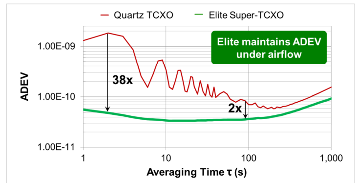
Best Allan Deviation (ADEV) in Still Air and Under Airflow
