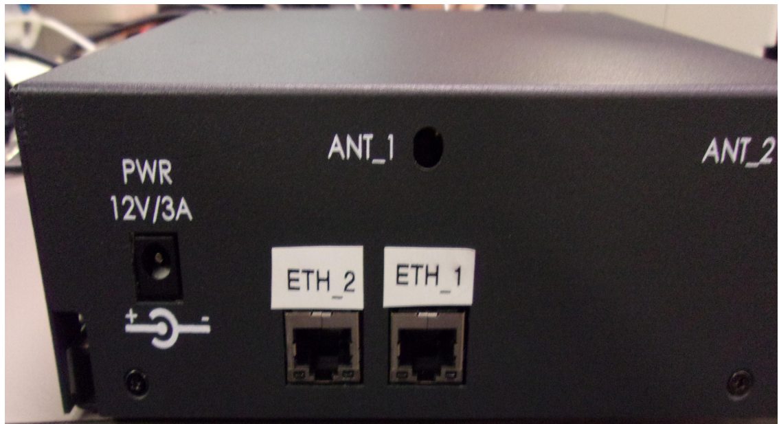
Figure 4. Correct ETH_1 and ETH_2 port markings on LS1012ARDB chassis
