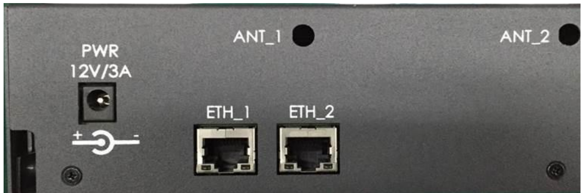
Figure 3. Incorrect ETH_1 and ETH_2 port markings on LS1012ARDB chassis
