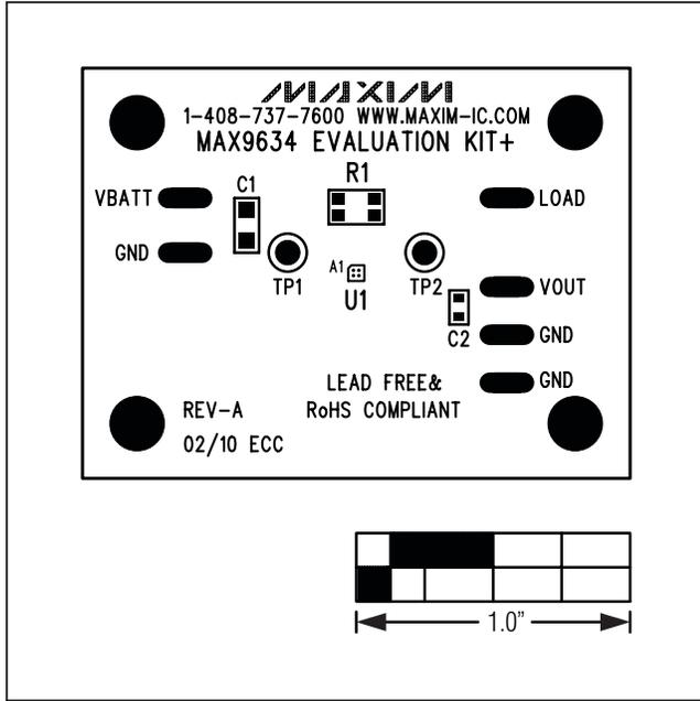
Figure 2. MAX9634 EV Kit Component Placement Guide—Component Side
