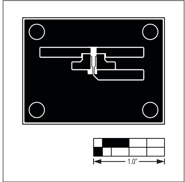
Figure 3. MAX9634 EV Kit PCB Layout—Component Side
