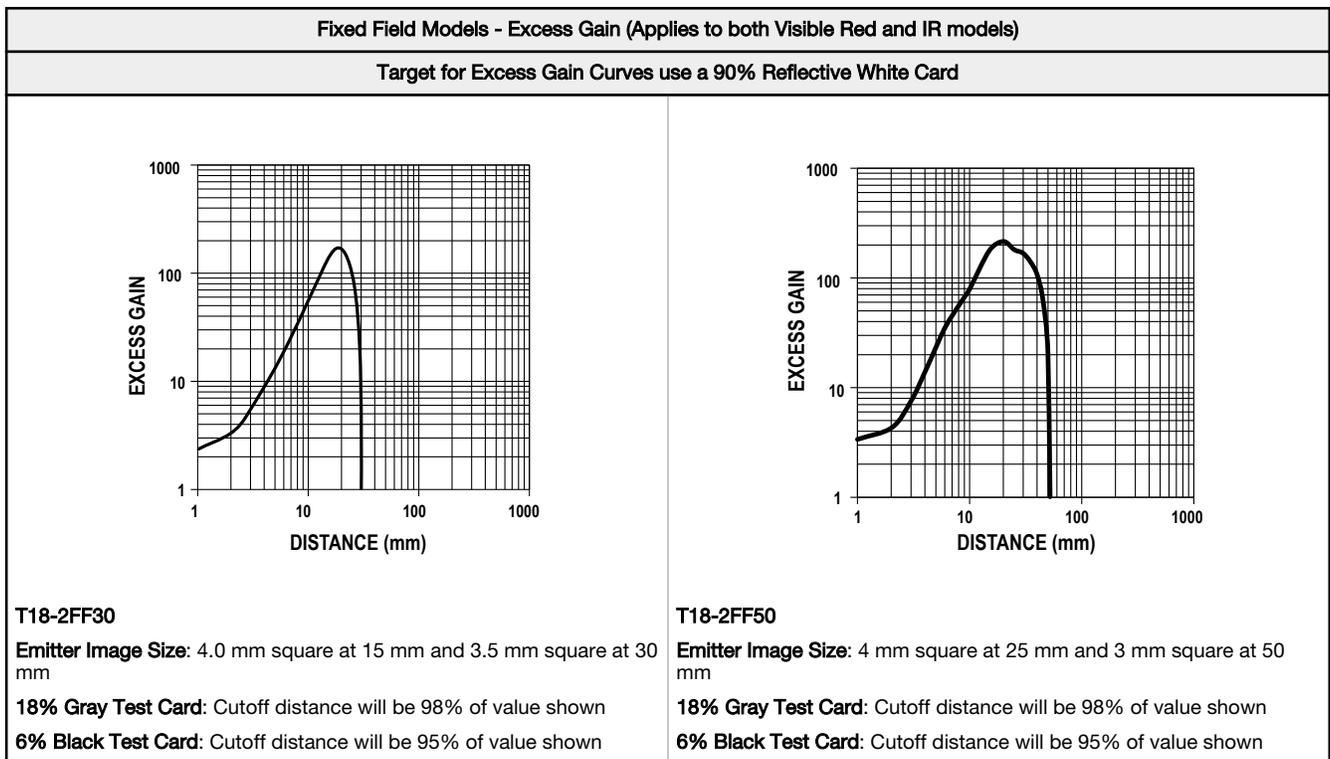
**Fixed Field Models - Excess Gain (Applies to both Visible Red and IR models)**
