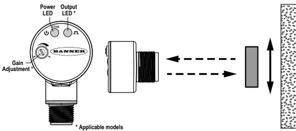
To install the T18-2 Epoxy Encapsulated Right-Angle Sensor:
