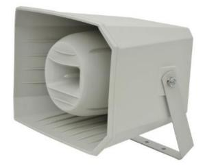
ABS full range horn speaker with 6.5" reverse mounted LF driver and front mounted 1" dome tweeter housed in an IP65 rated UV stabilised enclosure. Unlike standard outdoor horn speakers, this powerful unit has a full range output and is therefore suitable for background music as well as public address.
