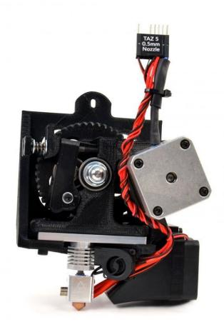
The new LulzBot TAZ Single Extruder Tool Head v2 has arrived. Built with an all metal LulzBot Hexagon Hot End, this tool head is capable of heating upto 300°C (572°F), so it easily handles standard filaments like HIPS, PLA, and ABS, as well as advanced filaments including heavy duty nylon, T-Glase, and polycarbonate, and aesthetic varieties of wood- and stone-like filaments.
