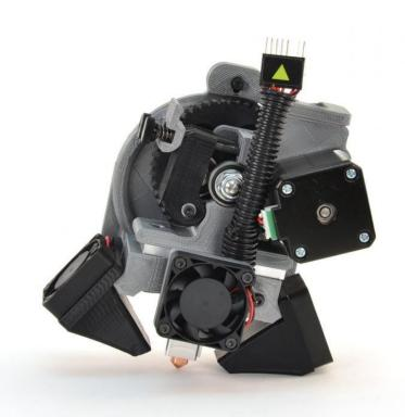
Bigger. Faster. Stronger. MOAR: The LulzBot TAZ MOARstruder Tool Head is a high output tool head with an extra-long heater block, dual print cooling fans, and a 1.2 mm diameter nozzle. These features enable high-speed printing and tough 3D printed objects.
