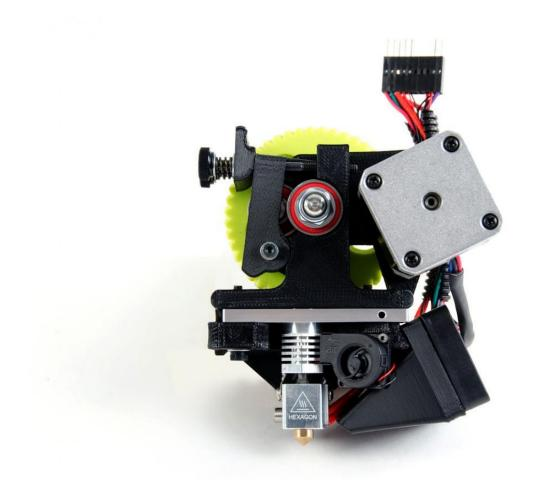
The LulzBot Mini Tool Head is an assembled complete assembly for your LulzBot Mini 3D printer. We use the popular Wade's Accessible Reloaded extruder & features the LulzBot Hexagon all-metal hot end (capable of temperatures up to 300C) mounted on our LulzBot Mini Extruder Mount. This tool head ships assembled, aligned and with all the connections terminated for ease of installation onto the LulzBot Mini.
