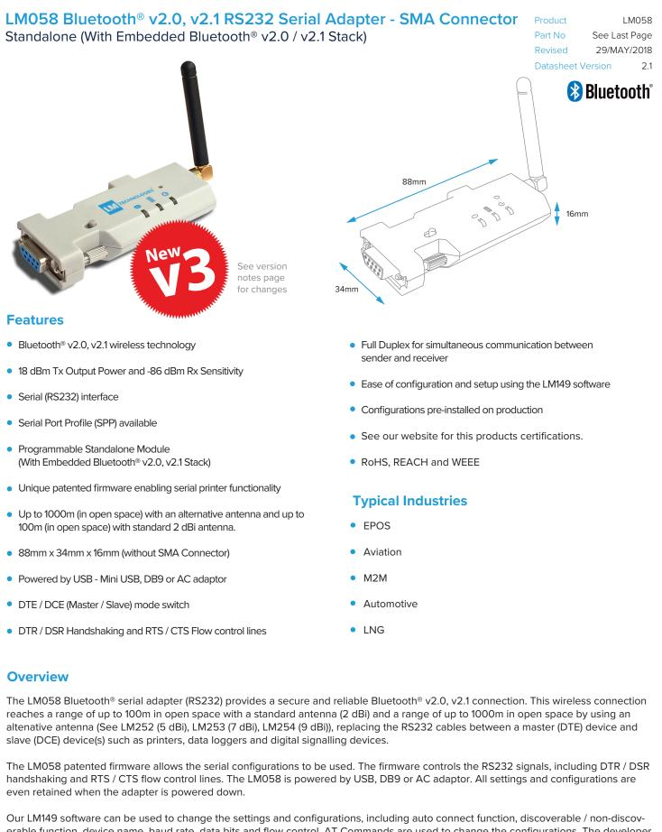
Our LM149 software can be used to change the settings and configurations, including auto connect function, discoverable / non-discoverable function, device name, baud rate, data bits and flow control. AT Commands are used to change the configurations. The developer is also able to configure and modify the settings of a remote LM058 from a local LM058. Customised configurations and settings can be preloaded to the LM058, simplifying the manufacturing and testing process.
