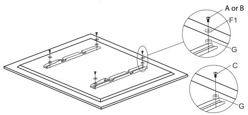
If the television has a curved back or includes an obstruction that may prevent the brackets from fitting flush to the back you can place the spacers (G) beneath the brackets to lift away from the back. The brackets can now be secured with screws A, B or C with the washers (F1) if necessary.
