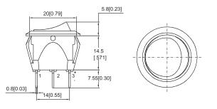
Panel cut out thickness: 0.8~3mm (0.031"~0.118")
