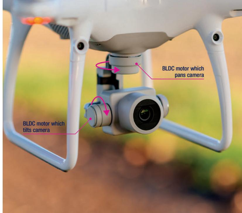
Figure 4. Example of a drone-mounted gimbal application for camera pan & tilt. (Source: STMicroelectronics)
