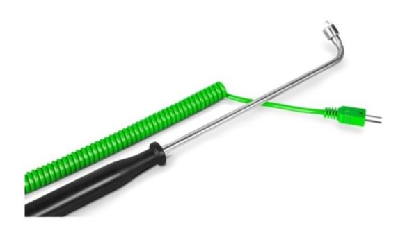
Stainless steel sheath with a moulded handle and 1.50metres of coiled extension cable terminated in a miniature thermocouple plug.
