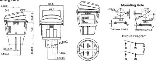
**Dimensions : Millimetres** Tolerances ±0.3mm
