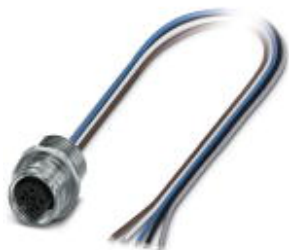
Flush-type connector, Universal, 5-position, Socket, straight, M12-Push-Pull, A-coded, Front mounting, M16 x 1.5, Individual wires, cable length: 0.5 m
