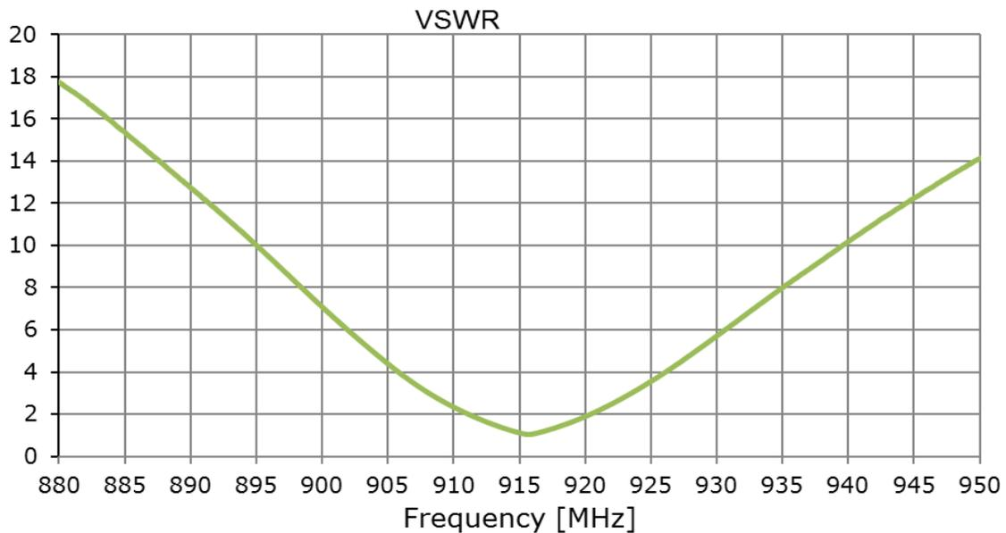
**Figure 3.** VSWR of 915 MHz ISM Band Antenna ILA.01
