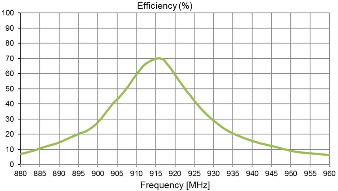
**Figure 4.** Efficiency of 915 MHz ISM Band Antenna ILA.01
