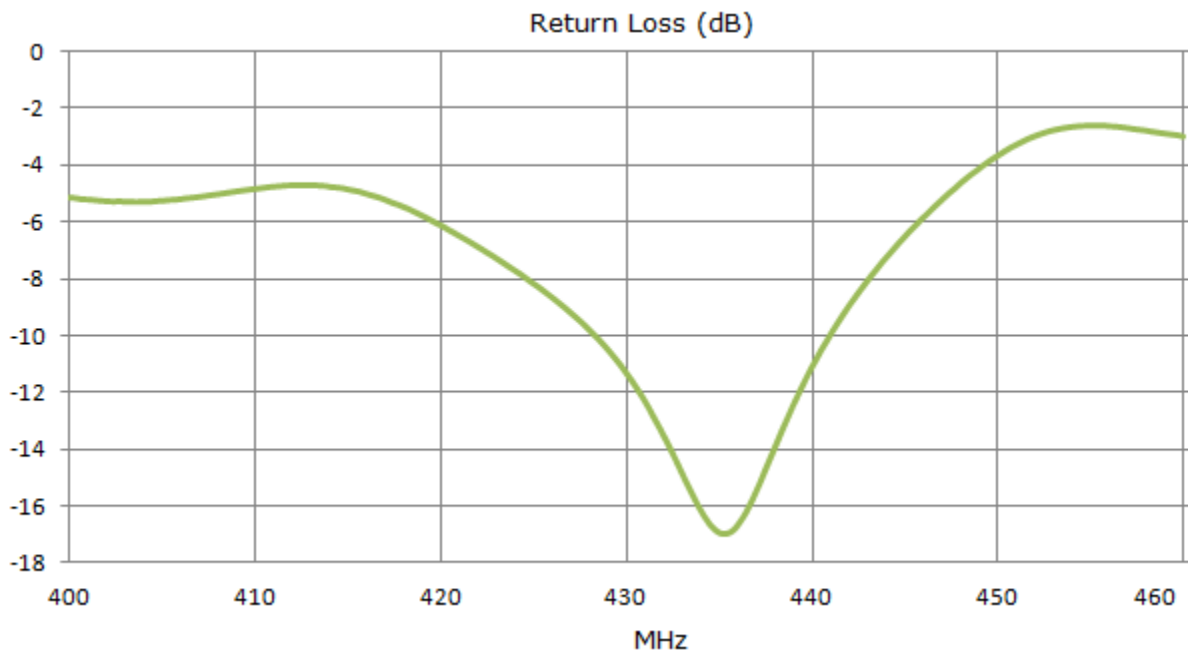
Figure 3 Return Loss of IS.01 Antenna on 30x30 cm metal plate.
