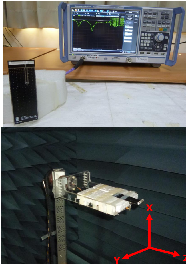
Figure 1. Impedance measurements (left hand) and peak gain, average gain, efficiency and radiation pattern measurements (right hand)
