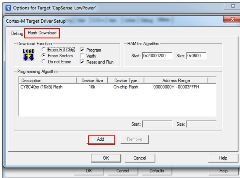
Figure 4-9. Flash Download Tab in Target Driver Setup
