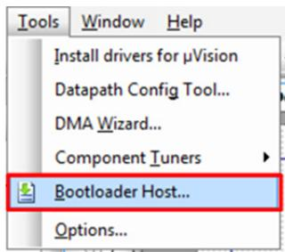
Figure 9-11. Open Bootloader Host Tool in All Programs
