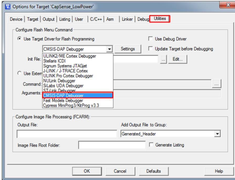
12. A programming algorithm must be added in the IDE to program PSoC 4. Click the **Settings** option. The **Cortex-M Target Driver Setup** window will open as shown in Figure 4-8. Go to the **Flash Download** tab and click the **Add** button as shown in Figure 4-9. Select the option corresponding to PSoC 4 in the programming algorithm.
