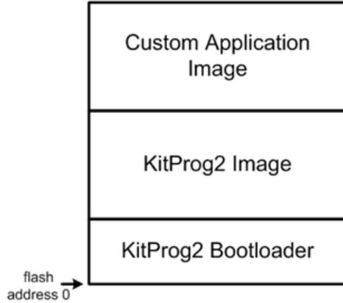
Figure 1-2 shows the KitProg2 flash architecture based on the concept of dual-image bootloading. If you are building custom applications for PSoC 5LP in KitProg2, only the ‘Custom Application Image’ flash area can be bootloaded with the corresponding *cyacd* file. The KitProg2 image cannot be bootloaded. It can only be restored to factory settings as described in [Restore PSoC 5LP Factory Program Using PSoC Programmer on page 74](#).
