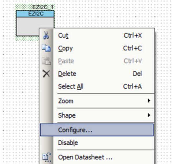
3. Configure the EZI2C Slave Component as shown in [Figure 7-6](#) and [Figure 7-7](#); then, click **OK**.
