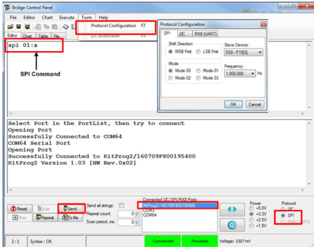
**Expected Output:** Sending a command word of 0x01, turns LED5 ON and a command word of 0x00 turns LED5 OFF.
