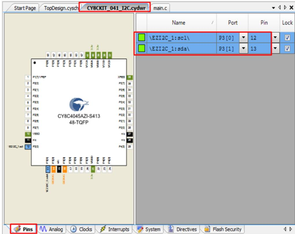
5. Place the following code in the *main.c* file. The code will enable the PSoC 4000S device with the BCP application using the EZI2C Slave interface.
