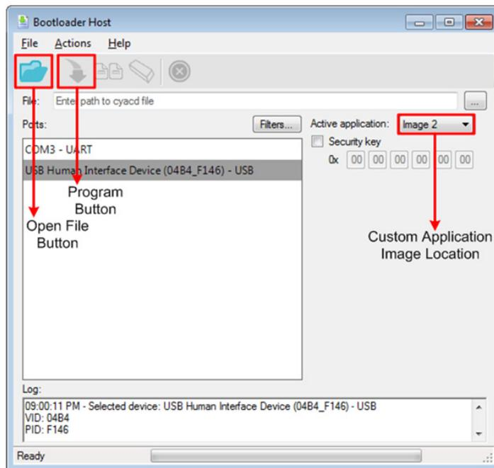
Figure 9-14. Select <Project\_Name\_2> .cyacd File from Bootloader Host Tool
