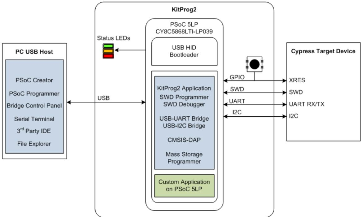
KitProg2 is an enhancement over KitProg. It follows the dual-image bootloading approach; the KitProg2 firmware is the first image and a custom application can be loaded as a second image. To learn more about the concept of dual-image bootloading, refer to application note [AN73854 – PSoC 3, PSoC 4, and PSoC 5LP Introduction to Bootloaders](#).
