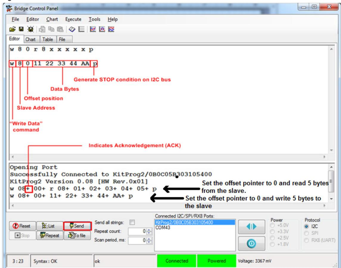
12. From the BCP, read back the five bytes of data just written from the I2C slave device with slave address 0x08. The log shows if the transaction was successful, as shown in [Figure 7-12](#).
