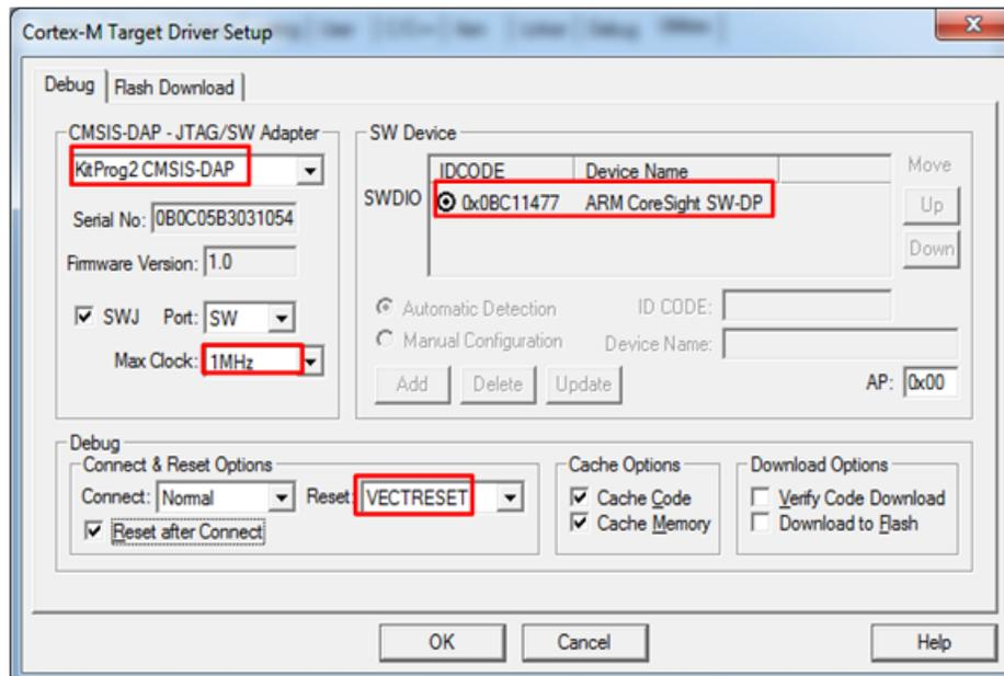
14. For debugging, go to the **Debug** tab and select the CMSIS-DAP Debugger as shown in Figure 4-11.
