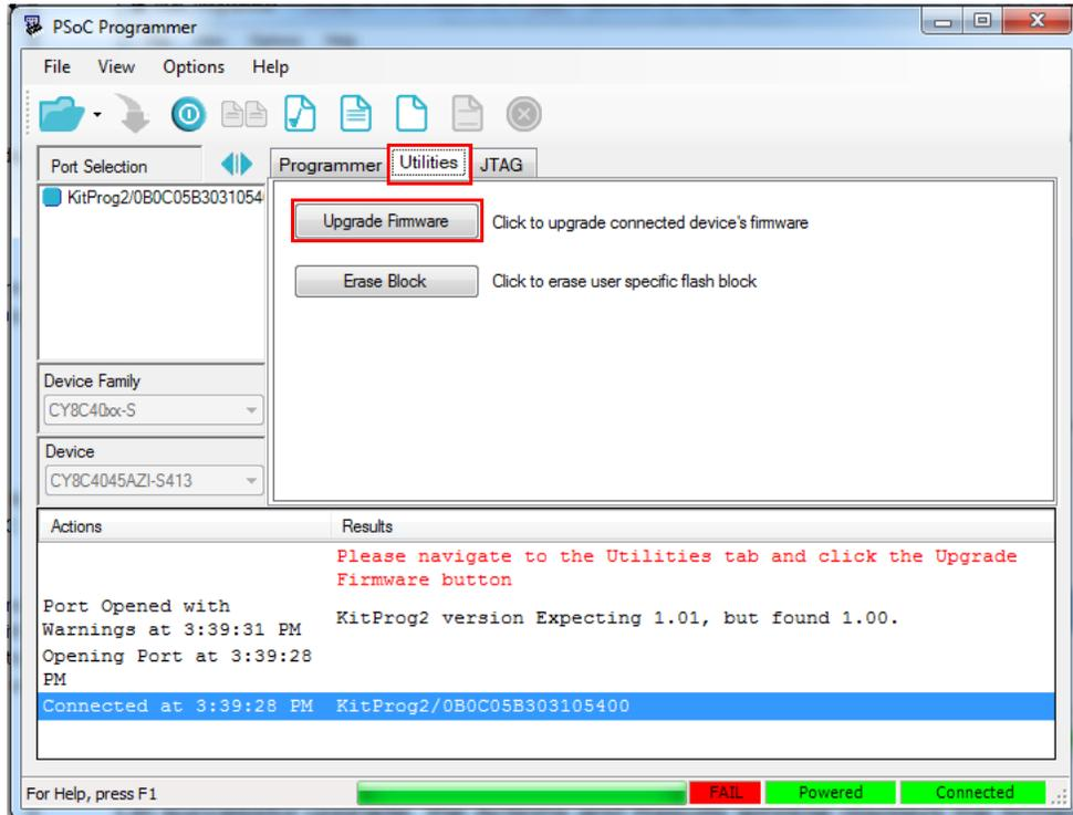
On successful upgrade, the Actions and Results window displays the firmware update message with the KitProg2 version, as shown in Figure 3-12.
