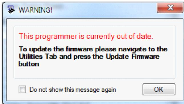
Click **OK** to close the window. On closing the warning window, the Actions and Results window displays: “Please navigate to the Utilities tab and click the Upgrade Firmware button”, as shown in Figure 3-11.
