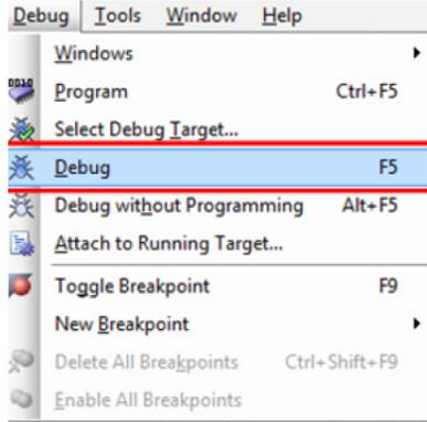
2. When PSoC Creator enters the Debug mode, use the buttons on the toolbar or keyboard shortcuts to debug your project.
