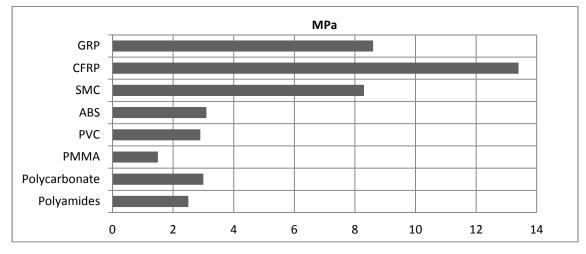
Average lap shear strengths of typical plastic-to-plastic joints (ISO 4587) (typical average values) Cured for 16 hours at 40°C and tested at 23°C. Pretreatment - Lightly abrade and alcohol degrease.
