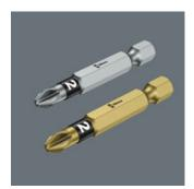
BTH- (extra-hard) and BTZ- (tough) bits have an additional tempered BiTorsion zone, which reduces the hardness of the shaft by about 20 % in comparison to the drive tip. This means that the peak loads that cause bit breakage and premature wear are absorbed in this zone — something which enhances the service life of the bits.
