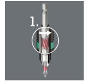
The torsion spring integrated into the unique BiTorsion holder absorbs lower levels of peak loads (Phase 1). Any overloading of this spring is effectively prevented by means of a supporting mechanism.
