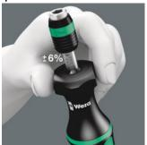
Simple setting of the required torque by hand. Easy-to-read scale value. Measurement accuracy is  $\pm$  6 % in accordance with the standard EN ISO 6789. Distinctly audible and noticeable excess-load signal when the pre-set torque is reached.
