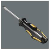
Wera makes its Kraftform handles from several materials with different properties. The core is made from a hardwearing plastic that holds the blade securely even when subjected to great forces. The yellow soft zones of the external mantle consist of a softer material with more friction resistance for high torque transfer. The black areas with a harder surface prevent the hand from sticking to the handle enabling you to adjust your grip more quickly. Non-roll feature
