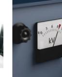
Our screwdrivers are tested for dielectric strength under a 10,000 volt load to make sure that their most important property, their insulation, has been exhaustively tested. Each individual Wera VDE screwdriver is subjected to this test to guarantee safe working up to 1,000 volts.
