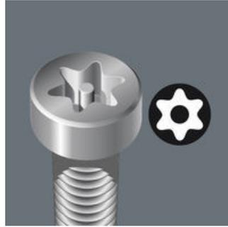
TORX® tools with a borehole prevent the unauthorised unfastening of safety screws. The screws contain a pin that protrudes into the drive profile so that “normal” TORX® tools cannot be used. This pin fits into the borehole of TORX® B0 tools allowing safety screws to be unfastened.
