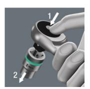
The ball lock holds the sockets and attachments securely, ensuring safe working. A changeover into predefined position is completed by simply pressing the release button - this is even the case in the 90° position.
