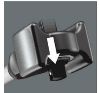
Changing the ratchet direction using a hardened push-through square drive ensures great resilience, since there is no susceptible switching mechanism that could be damaged by hammer blows. This is far more robust than a forward/reverse switch.
