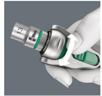
All Zyklop Speed ratchets feature a thumbwheel that can be used to quickly and easily switch between clockwise and anticlockwise rotation, at any position. No complicated handling, no loss of time!
