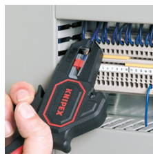
Stripping in confined areas
