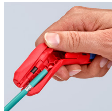
Stripping of a data cable
