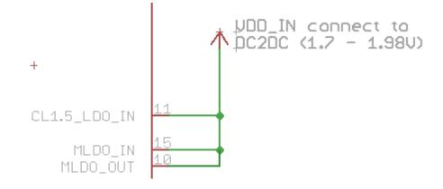
Mixed DC2DC-V<sub>BAT</sub> system (Maximum RF output power and optimum system power, but requires routing of V<sub>BAT</sub>):
