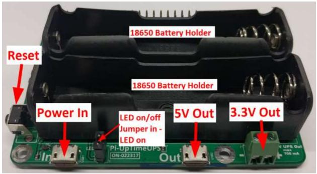
Please make sure power is plugged into Power In port shown above, and NOT the Raspberry Pi Power In.
