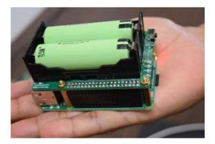
to the Raspberry Pi. Pi-UpTimeUPS provides power mobility for the Raspberry Pi.
