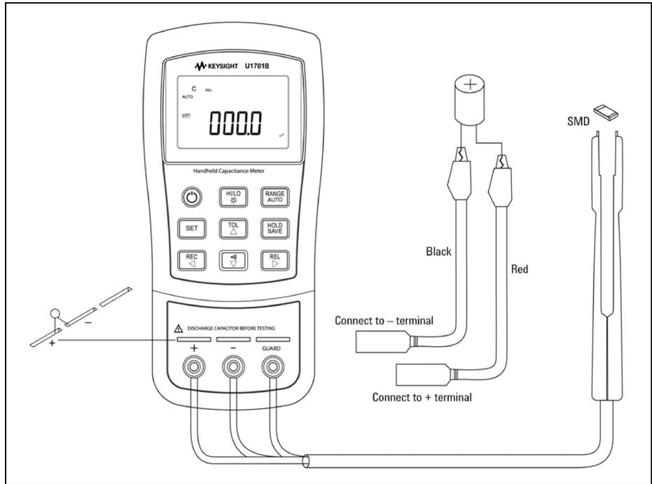
Figure 2-8 Capacitance measurement
