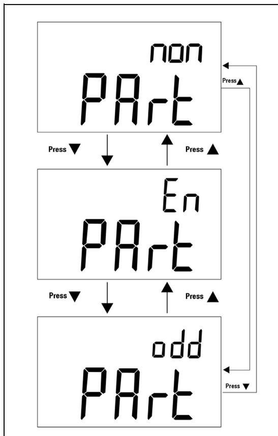
**Figure 3-2** Parity check setup for remote control
