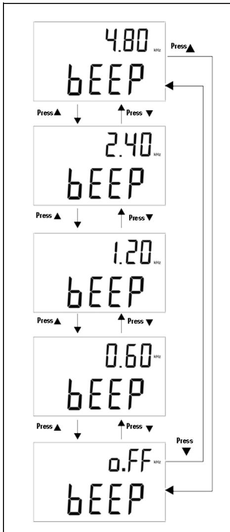
**Figure 3-6** Driving frequency of Beeper setup
