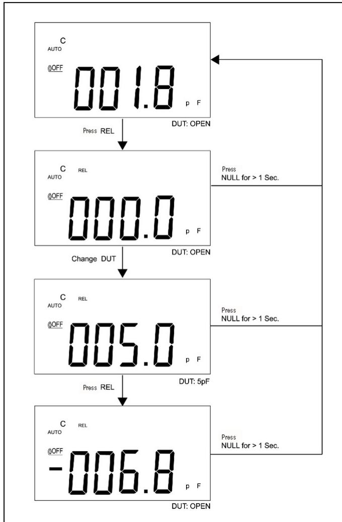
**Figure 2-3** Relative (Zero) operation
