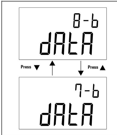
**Figure 3-3** Data bit setup for remote control
