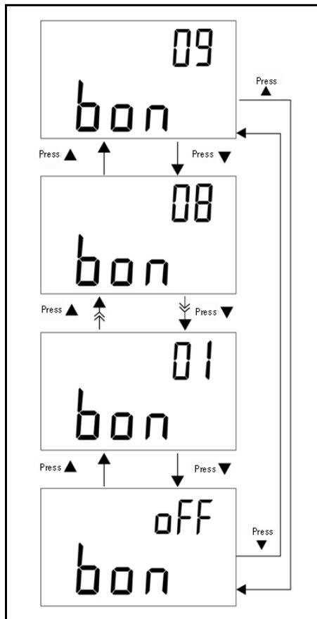
Figure 3-11 Brightness level for ON state
