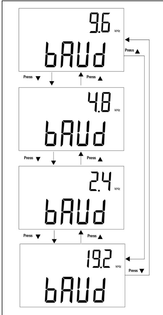
**Figure 3-1** Baud rate setup for remote control
