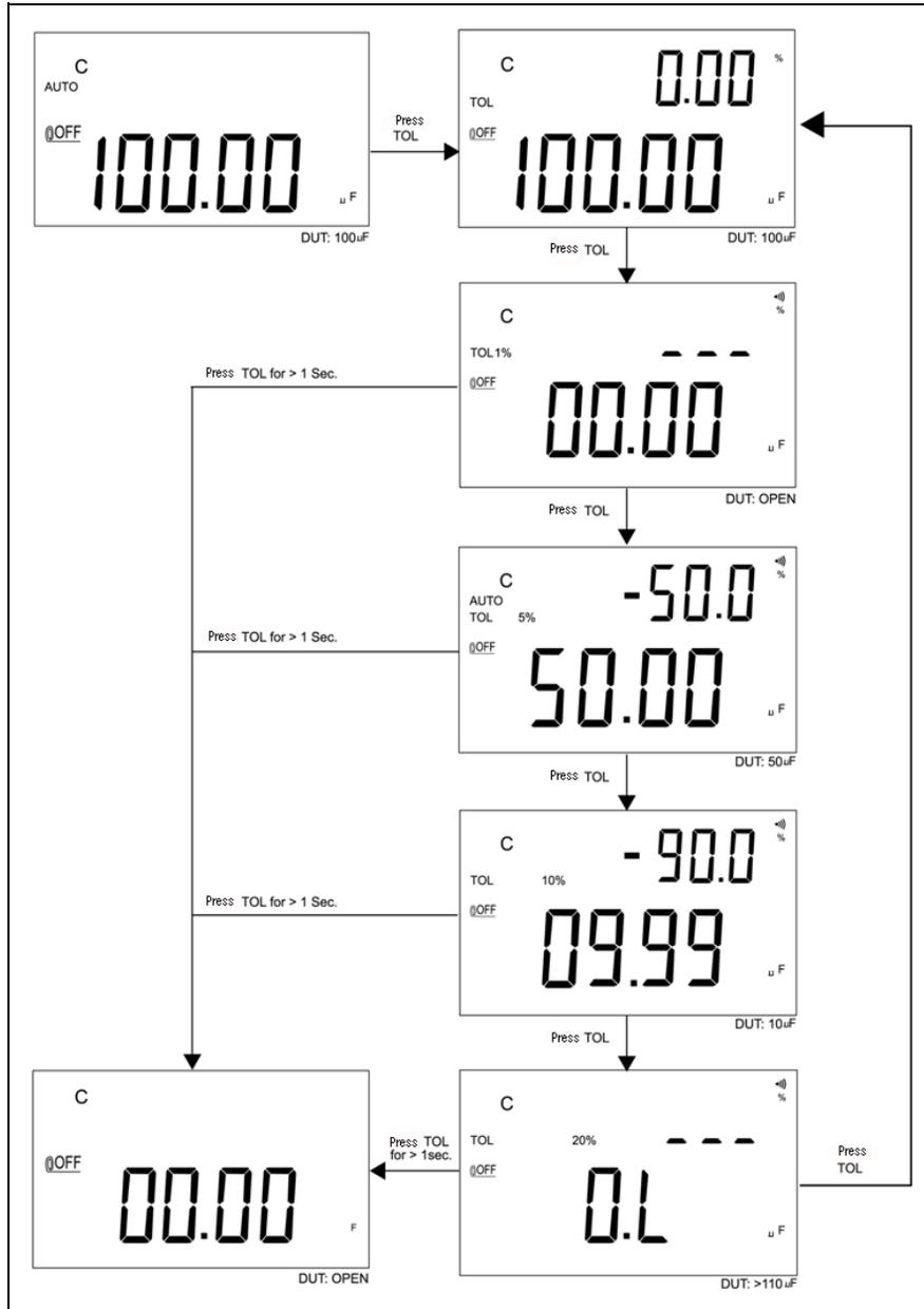
Figure 2-4 Tolerance operation
