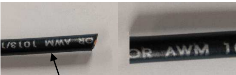
Jacket End Cut Straight or with 10° Maximum Angle
