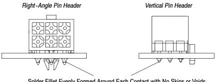
Solder Fillet Evenly Formed Around Each Contact with No Skips or Voids (No Solder on Boardlocks)
