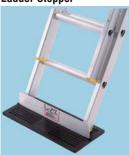
The ladder stopper is an aluminium T piece bonded into a 11mm vulcanised rubber base complete with a 2mm tread top and bottom. Designed for extra grip even in the wet.
