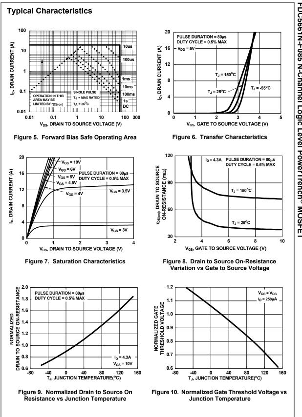
FDC5661N-F085 N-Channel Logic Level PowerTrench<sup>®</sup> MOSFET
