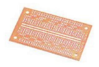
Board was designed for ICs to straddle center of board. There are 26 rows designated for IC pin connections with 2 additional connections for IC with added connections toward outer edges of board. Board measures 115/16" x 111/16" x 3/32".
