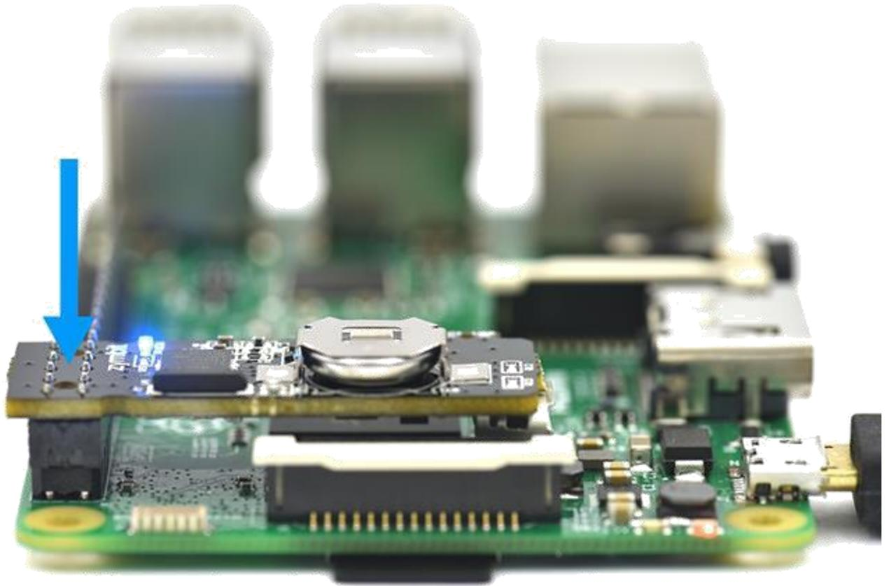
Fit the Zymkey 4i with battery facing upwards. Be sure the black connector is properly aligned with the first 10 GPIO pins and that pressed firmly down onto the header. If missaligned, this could cause damage to the Zymkey and/or your Raspberry Pi. Your Zymkey should fit relatively snug and maintain a tight interference fit around the pins.
